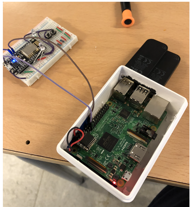
Figure 3. Arduino-based sound measurement sensor (left background) packaged with Raspberry PI (right foreground) for IoT deployment.
